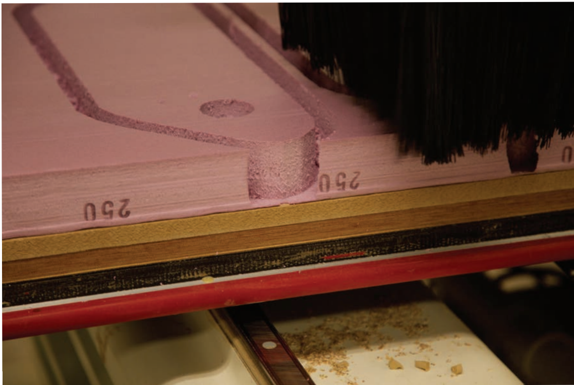
Figure 19. Foam Cut. Image shows how individual pieces are still connected to the larger sheet. This allowed for me to transport all of the small pieces more easily.
