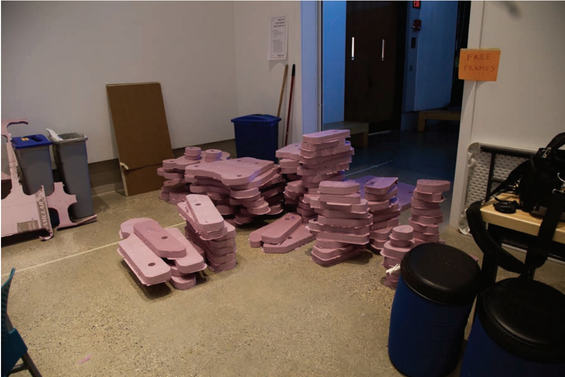
Figure 23. The foam pieces stacked and prepared for full assembly. They broke out of the larger sheet easily.
