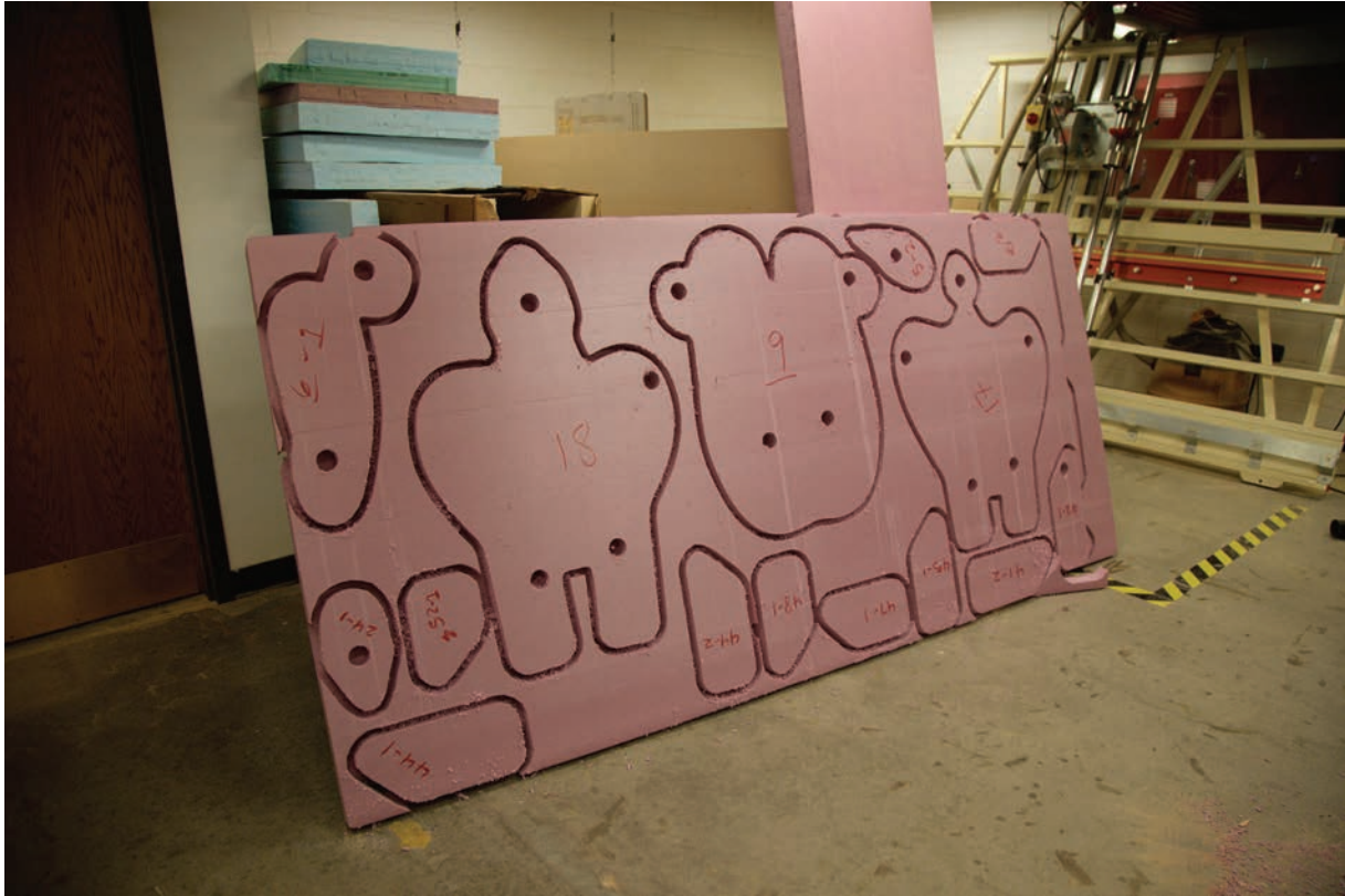
Figure 21. Another fully cut sheet. The numbers written on each piece exhibit the stacking order.
