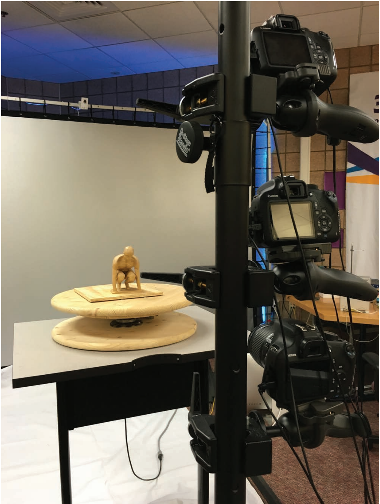
Figure 9. 3D Scanning the simplified clay mock up. Scan took place in the Duderstadt Center.
