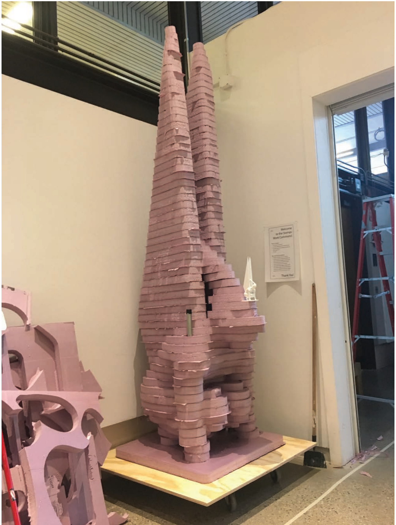
Figure 28. Final 3D Print, and Assembled foam model. Next step is foam smoothing and clay application.
