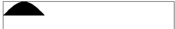
Figure 3. Envelope for grain shaping in a 4.0 surround system, in this case a Gaussian envelope covering only a \frac{1}{4} of the entire duration of the rotation time window.
