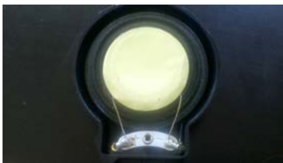
Figure 4. Tactile transducer attached to percussion instrument surfaces in fcremaperc .
