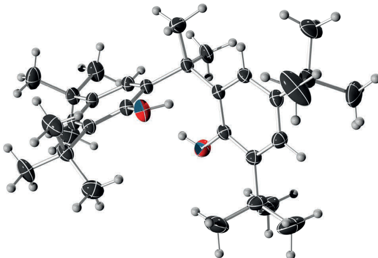
Figure 4. ORTEP ellipsoid-and-stick model of the single-crystal X-ray structure of 6,6'-(propane-2,2-diyl)bis(2,4-di- tert -butylphenol) ( 1 ). Color code: C black, H gray, O red. 32,33
